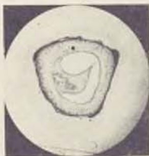
Cross section of rodent bone which was mounted in room temperature setting encapsulant because of its fragile nature before sectioning.
