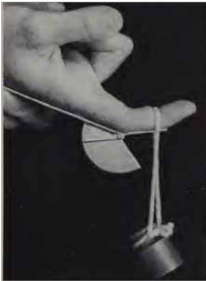
Fig. 1. Brand's method to obtain torque-angle measurement is suggested for the hand to be positioned so that a hanging weight of e.g. 250 g is pulling at right angles to a segment of a finger and at a finger crease. Alternatively, the weight may hang over a pulley wheel so that the string is horizontal and the hand is more easily positioned [5].
