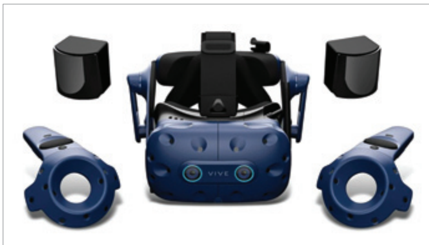
Fig. 1. HTC® Vive Pro Eye VR headset with controllers and base stations [31].
